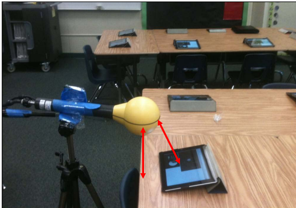
Photo 10 – Room 7, typical instrument antenna placement for measurements. Approximately 10 to 12 inches from device, representing likely location of a child's head in relationship to the device.
